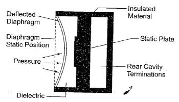
Fig. 13.29 Capacitive Pressure Transducer
