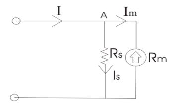
Basic Ammeter Circuit
