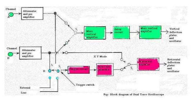
The two separate input signals can be applied to single electron gun with the help of electronic switching it Produces a dual trace display .Each separate vertical input channel are uses separate attenuators and pr-amplifier stages, so the amplitude of each signal can be independently controlled. Output of the pramplifiers is given to the electronic switch, which passes one signal at a time into the main vertical amplifier of the oscilloscope.
