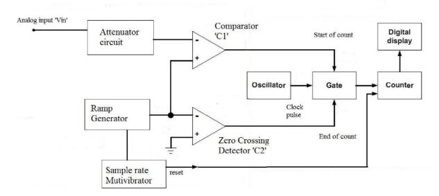
At the start of the measuring cycle, a ramp voltage is initiated; this voltage can be positive going or negative going. The negative going ramp, shown in the fig. is continuously compared with the unknown input-voltage.
