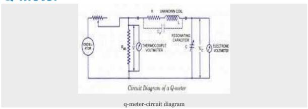
We know that every inductor coil has a certain amount of resistance and the coil should have lowest possible resistance. The ratio of the inductive reactance to the effective resistance of the coil is called the quality factor or Q-factor of the coil.
