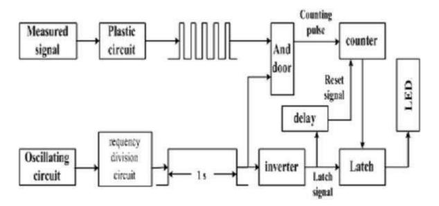
Fig .1 Digital frequency meter principle diagram
