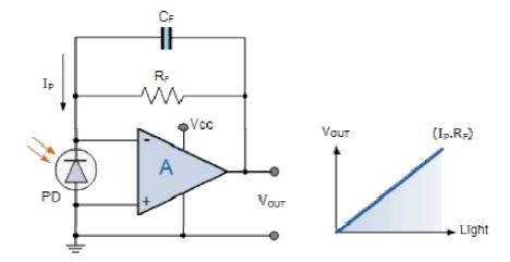
**Photodiodes** are very versatile light sensors that can turn its current flow both "ON" and "OFF" in nanoseconds and are commonly used in cameras, light meters, CD and DVD-ROM drives, TV remote controls, scanners, fax machines and copiers etc, and when integrated into operational amplifier circuits as infrared spectrum detectors for fibre optic communications, burglar alarm motion detection circuits and numerous imaging, laser scanning and positioning systems etc.
