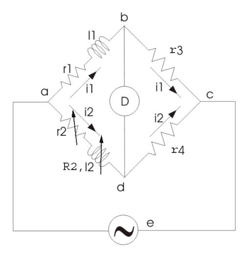
In this bridge the arms bc and cd are purely resistive while the phase balance depends on the arms ab and ad.
