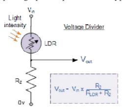
Connecting a light dependant resistor in series with a standard resistor like this across a single DC supply voltage has one major advantage, a different voltage will appear at their junction for different levels of light.
