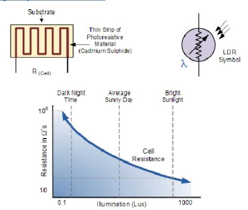
The most commonly used photoresistive light sensor is the **ORP12** Cadmium Sulphide photoconductive cell. This light dependent resistor has a spectral response of about 610nm in the yellow to orange region of light. The resistance of the cell when unilluminated (dark resistance) is very high at about  $10M\Omega$ 's which falls to about  $100\Omega$ 's when fully illuminated (lit resistance).
