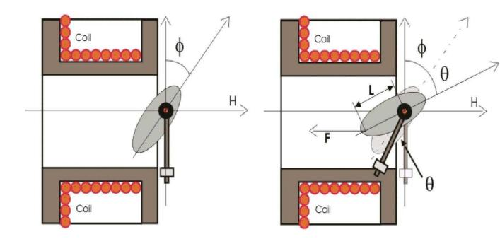
Working of Moving Iron Instrument
