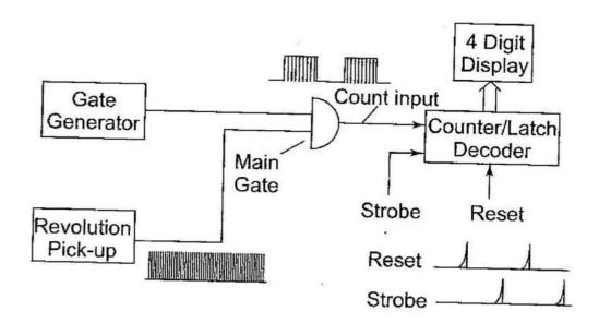
Basic Block Diagram of a Digital Tachometer
