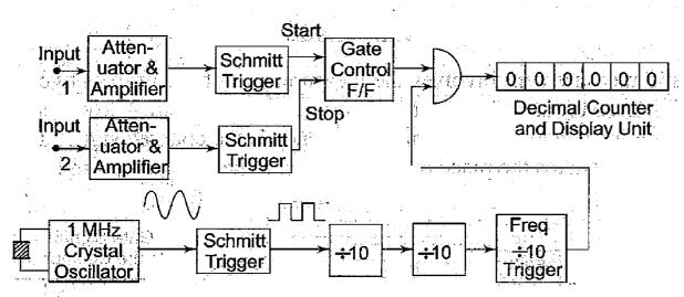
Fig. Basic Block Diagram of Time Measurement
