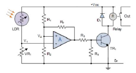
In this basic dark sensing circuit, the light dependent resistor LDR1 and the potentiometer VR1 form one adjustable arm of a simple resistance bridge network, also known commonly as a *Wheatstone bridge*, while the two fixed resistors R1 and R2 form the other arm. Both sides of the bridge form potential divider networks across the supply voltage whose outputs V1 and V2 are connected to the non-inverting and inverting voltage inputs respectively of the operational amplifier.
