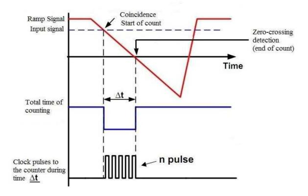
The sample-rate multi-vibrator[MV] determines the rate at high the measurement cycle are initiated. The sample-rate circuit provides an initiating pulse for the ramp generator to start its next ramp voltage. At the same time, a reset pulse is generated which returns all the DCUs o their zero state, removing the display momentarily from the indicator tubes.
