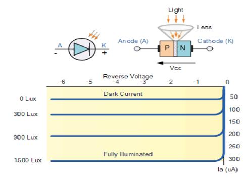
When used as a light sensor, a photodiodes dark current (0 lux) is about 10uA for geranium and 1uA for silicon type diodes. When light falls upon the junction more hole/electron pairs are formed and the leakage current increases. This leakage current increases as the illumination of the junction increases.
