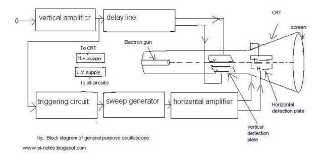
The oscilloscope can be adjusted so that repetitive signals can be observed as a continuous shape on the screen. A storage oscilloscope allows single events to be captured by the instrument and displayed for a relatively long time, allowing human observation of events too fast to be directly perceptible.
