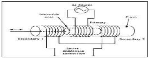
Similarly , When movable core moves towards coil  $S_1$ ,  $E_1 > E_2$  and  $V_0 = E_1 - E_2$  and is in phase with  $E_1$ .
