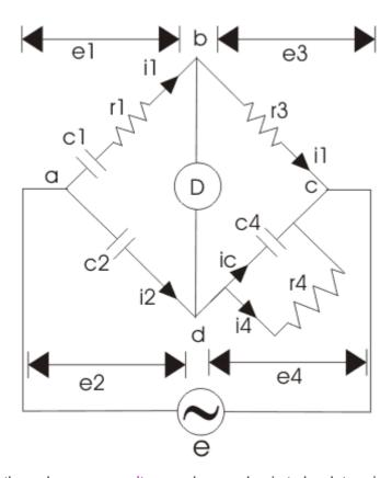
Here, c<sub>1</sub> is the unknown <u>capacitance</u> whose value is to be determined with series <u>electrical</u>
